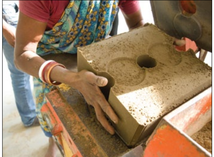
A local woman makes a brick of densely packed earth at a small outdoor facility in the village of Langleswar, in the state of Orissa, India. These building bricks are environmentally friendly and are being used on homes built by CRS to be flood resistant.
